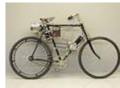
1902 - Clément Autocyclette 143 cc with A. C. KREBS intake regulation.
