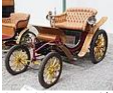
Side view of the 1900 Clément-Panhard Phaeton (VCP), 765cc 3,5cv, achieving a top speed of 35kmh.
