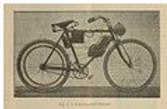
1901 - The Clément autocycle with the removable motor derived from the Krebs engine of the Clément-Panhard Car.
